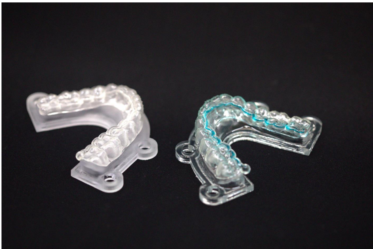
Two prototypes of "Active Aligners" equipped with antibacterial diffusers. The one on the left represents the transparent aligner prototype in its final appearance. The prototype on the right contains a blue liquid highlighting the innovation: a 3D-printed microchannel system.
